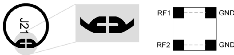
Figure 3-13 Small loop antenna (8 mm) designed for shunt connection. Impinj Button™ shown (L) with antenna trace detail (C) and corresponding chip/antenna connections (R)
