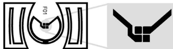
Figure 3-6 Antenna designed for single-ended connection. Satellite antenna shown (L), with antenna trace connection detail (R). Note the diagonal pad contacts between RF1 and GND.
